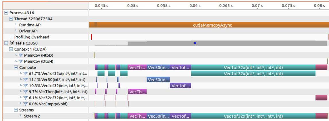
Along the top of the view is a horizontal ruler that shows elapsed time from the start of application profiling. Along the left of the view is a vertical ruler that describes what is being shown for each horizontal row of the timeline, and that contains various controls for the timeline. These controls are described in [Timeline Controls](#)
